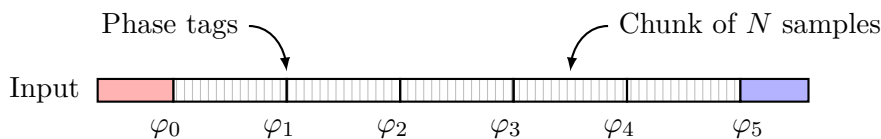
Figure 3.3 Graphical representation of the input samples for the work function of the fine phase and frequency correction block (shown in listing 3.2). Roughly every N samples there is a tag containing the information of the phase error (computed using the cross correlation peak). The white ‘chunks’ of samples can be corrected using their respective left and right tag values. The samples in the red chunk need phase information from the previous block processing. The samples in the blue chunk need a phase information from the future, which is not attainable. Thus for the blue chunk the frequency estimate of the previous chunk is used.
